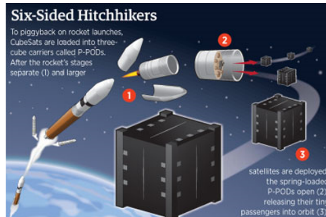
Figure 1.7: Launch sequence of deploying CubeSats during a larger commercial mission [16]
